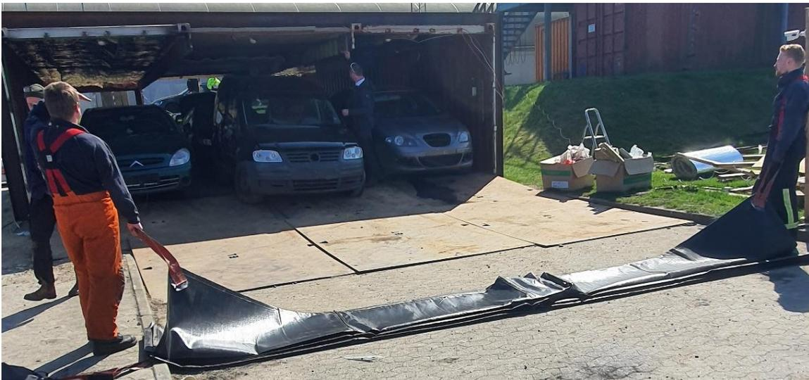
*Figure 3.8: Standard Bridgehill Car Fire Blanket unrolled on the ground ready for use*
