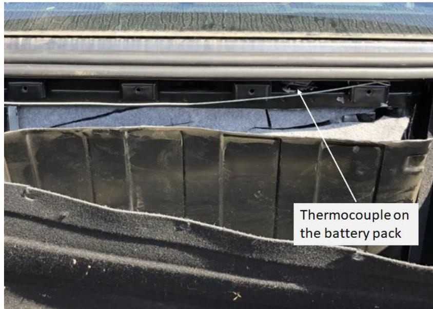
*Figure 3.7: Thermocouple placement on the battery pack*
