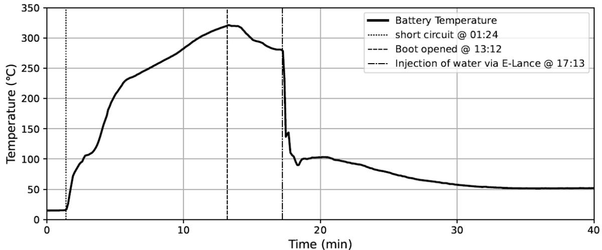
Figure 3.15: Battery compartment temperature during experiment 2
