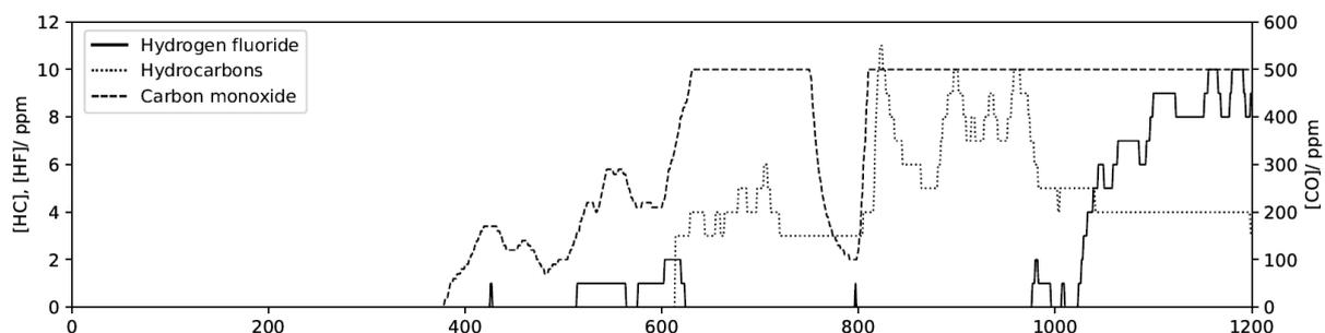
Figure 3.27: Live measurements of HC, HF and CO concentrations from experiment 6
