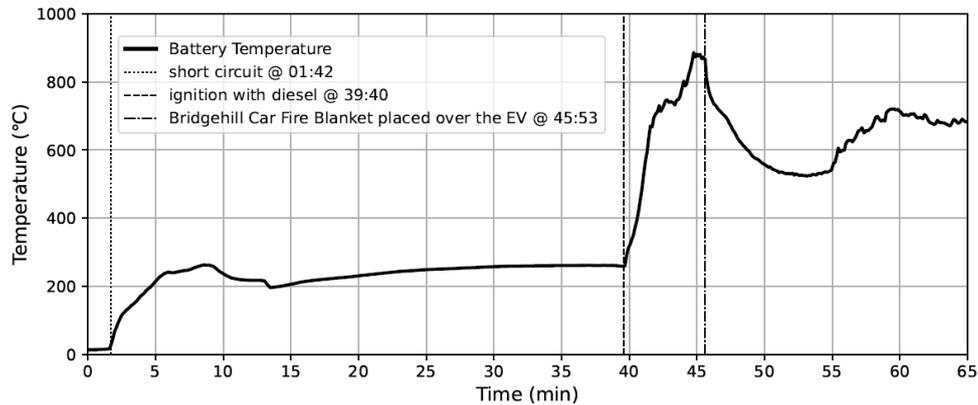
Figure 3.10: Battery compartment temperature during experiment 1
