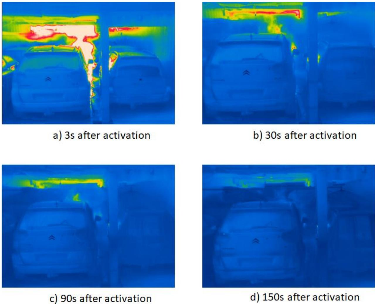
Figure 3.26: Thermal images of the surrounding after sprinkler activation; a) 2 sec after activation, b) 30 sec after activation, c) 90 sec after activation, d) 150 sec after activation
