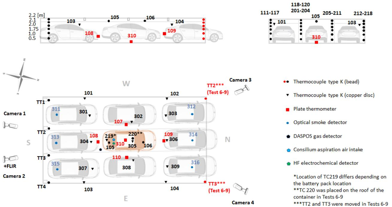
Figure 3.5: Arrangement of the measuring devices and cameras
