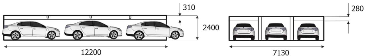
Figure 3.2: Dimensions of the experimental set-up (dimensions in millimeters)
