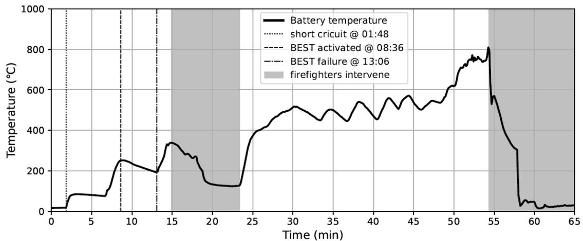
Figure 3.17: Battery compartment temperature during experiment 3
