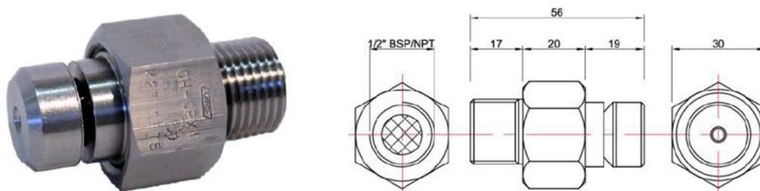
Figure 3.24: VID Fire-Kill low pressure water mist nozzle (left) and the dimensions (right)
