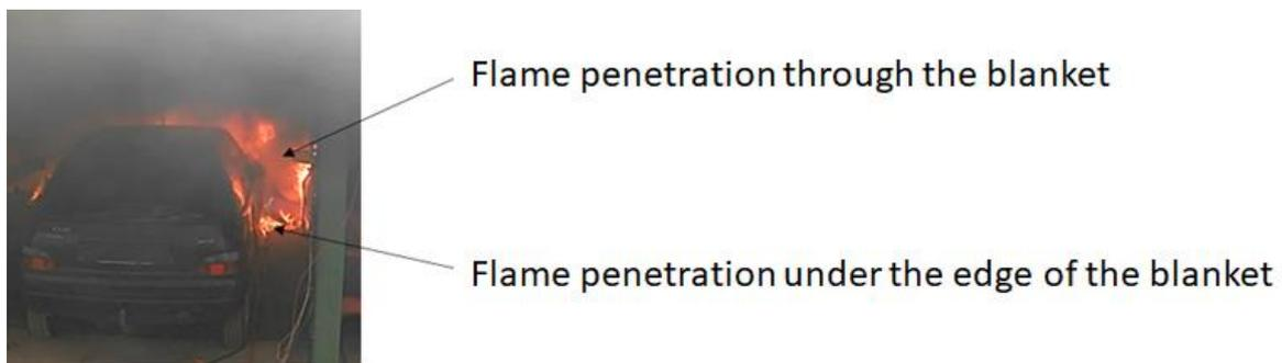
Figure 3.11: Flame penetration through the fire blanket
